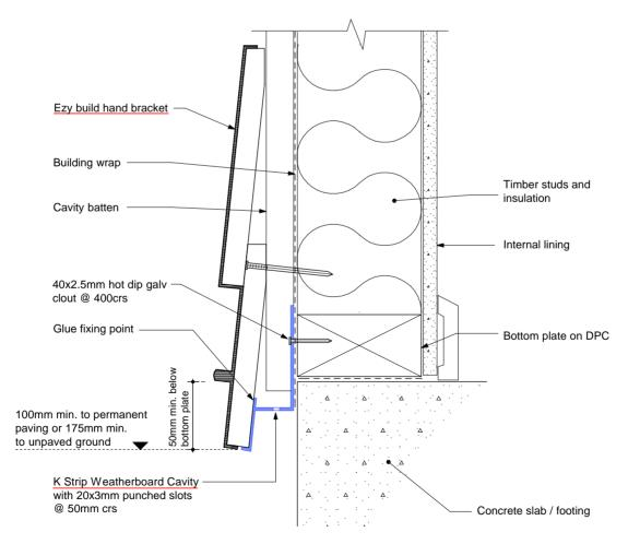
STEP 3 - Use hand bracket to fit remaining weatherboards
