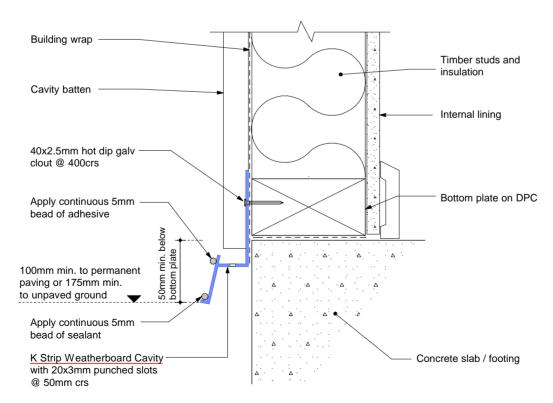
STEP 1 - Fix K-Strip Weatherboard Cavity- Apply glue and sealant
