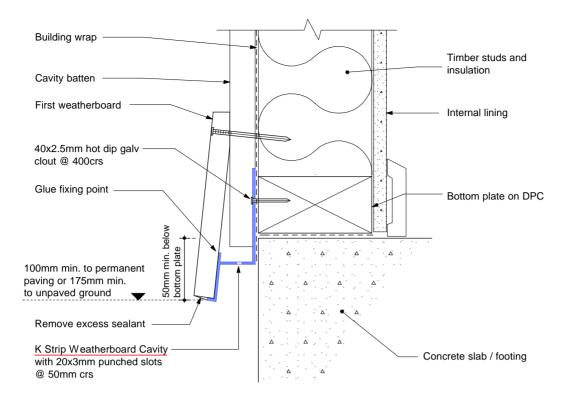
STEP 2 - Fix first weatherboardRemove excess sealant
