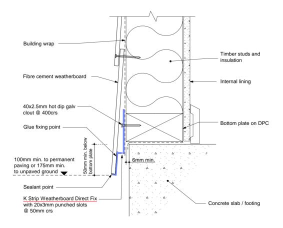
STEP 2 - Fix first weatherboard - Remove excess sealant
