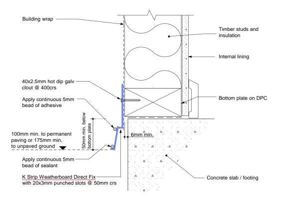
STEP 1 - Fix K-Strip Weatherboard Direct Fix- Apply glue and sealant
